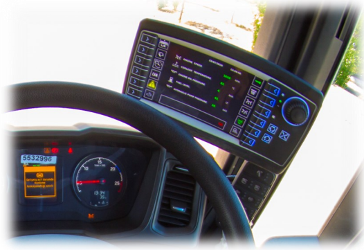
CAN BUS CONTROL UNIT
