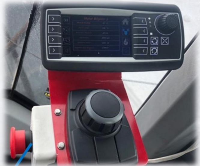
CAN Communication Enabled Ergonomic Control Unit
