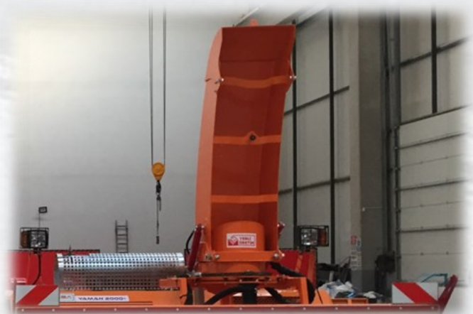
250° Rotation Capable High Discharge Chimney
